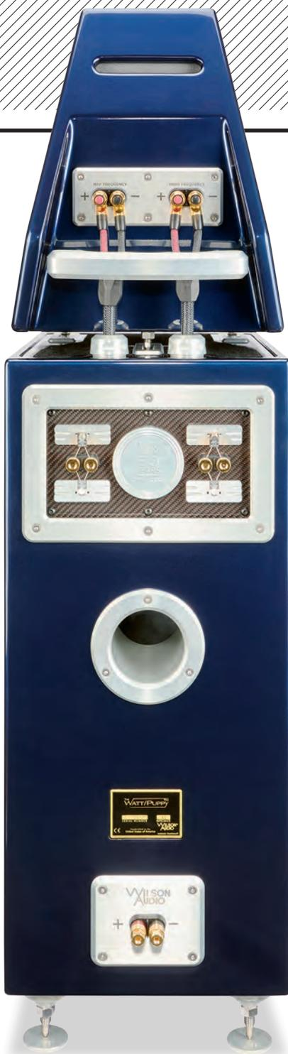
**LEFT:** Rear view shows lower-to-upper cabinet connections, rear-firing port, midrange vent and access to 'protection' resistors. The crossover is in the main cabinet and does not support bi-wiring
